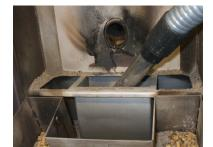
Fig. 27 - Burning pot box cleaning
