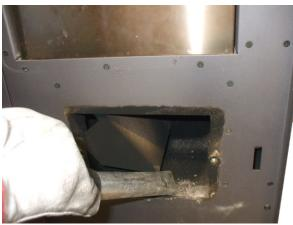
Fig. 31 - Fume chamber cleaning
