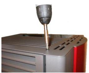
Fig. 15 - Upper screws removal
