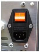
Fig. 43 - Electric socket with master switch
