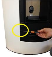
Fig. 74 - Loosen the bottom screw
