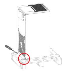
Fig. 1 - Bracket removal
