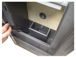
Fig. 58 - Burning pot box cleaning
