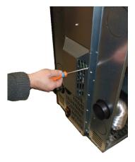
Fig. 89 - Rear panel removal
