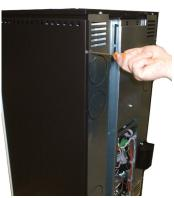
Fig. 62 - Removing the rear screw
