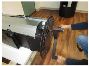
Fig. 47 - Remove the three-legged stand
