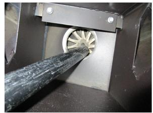
Fig. 99 - Vacuum out the ash
