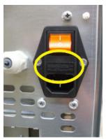
Fig. 106 - Shutter with fuses to remove
