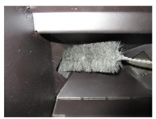
Fig. 103 - Cleaning with pipe cleaner 4
