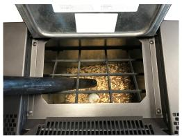
Fig. 91 - Hopper and auger cleaning
