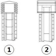
Fig. 4 - Anti-wind chimney pots
