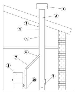
Fig. 5 - Chimney components
