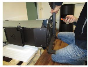
Fig. 48 - Secure the bench pedestal
