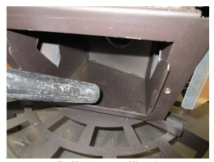
Fig. 98 - Vacuum out the ash
