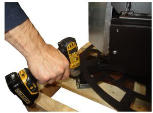
Fig. 34 - Bracket removal
