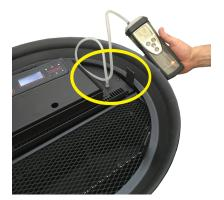
Fig. 68 - Digital pressure switch connection
