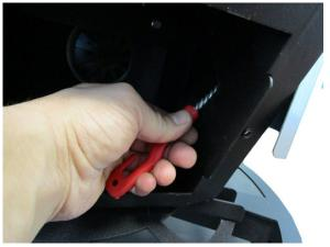
Fig. 102 - Cleaning with pipe cleaner 3
