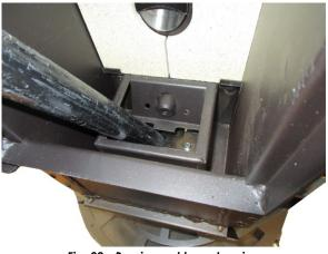
Fig. 89 - Burning pot box cleaning
