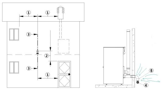
Fig. 7 - Air inlet for sealed-chamber installation
