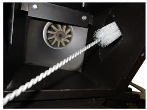
Fig. 100 - Cleaning with pipe cleaner 1
