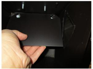
Fig. 97 - Flue gas deviator removal
