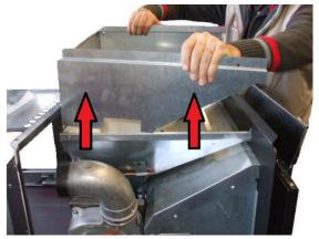
Fig. 60 - Casing removal
