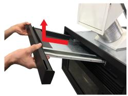
Fig. 34 - Removing drawer 1
