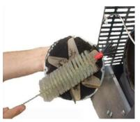
Fig. 50 - Exhaust fan cleaning: stage1
