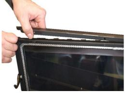
Fig. 56 - Door profiles removal
