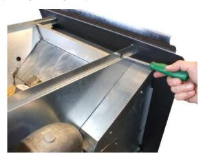
Fig. 59 - Unnscrew casing screws
