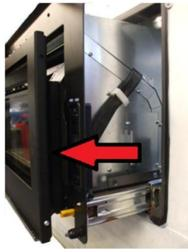
Fig. 58 - Insert extraction
