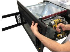
Fig. 37 - Securing the front panel
