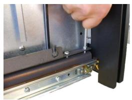
Fig. 14 - Insert fixing front screw
