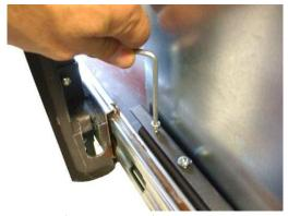
Fig. 20 - Insert fixing rear screw
