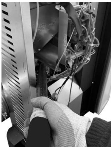
Fig. 108 - Czyszczenie wentylatora (Atena³ Plus 12/14 - Duke 12/14 At - Saba 12/14)
