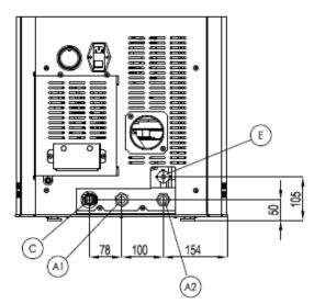
Fig. 20 - Plumbing connection
