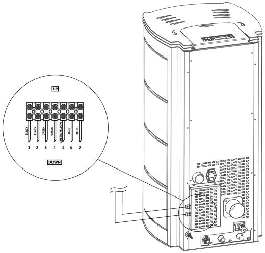
Fig. 36 - Electrical thermostat connection
