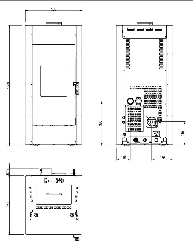
Fig. 9 - Idron 11 dimensions
