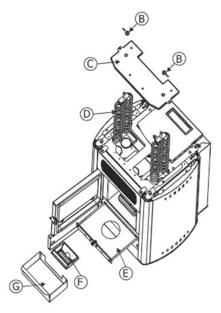
Fig. 41 - Cleaning the pipe unit, turbulators and lower compartment (Aquos 15-22-22 H2O / Ibis 15-22-22 H2O / Idron 15-22-22 H2O)
