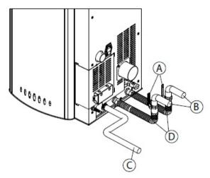
Fig. 21 - Plumbing connection
