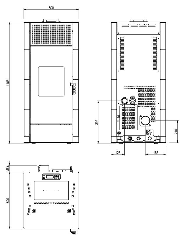
Fig. 10 - Idron 15 - Idron 22 - Idron 22 H2O dimensions
