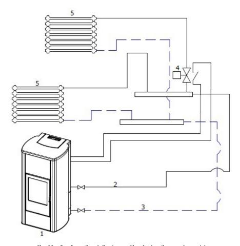
Fig. 29 - Configuration 1 (factory setting for heating version only)
