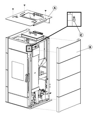
Fig. 16 - Metal sides insertion
