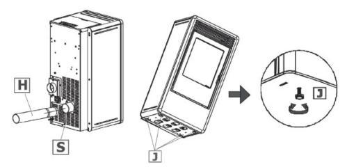
Fig. 14 - 1. Turn the feet clockwise to lower the stove - 2. Turn the feet counterclockwise to raise the stove
