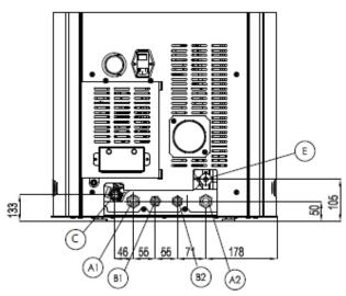
Fig. 19 - Plumbing connection
