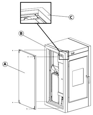
Fig. 17 - Metal sides insertion
