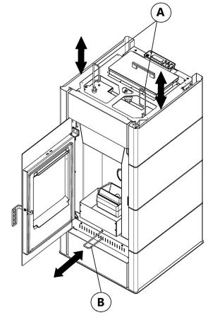
Fig. 39 - Cleaning the internal pipe unit using scrapers (Aquos 15-22-22 H2O / Ibis 15-22-22 H2O / Idron 15-22-22 H2O)
