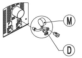
Fig. 22 - End piece with a filling tap (D) and pressure gauge (M) (Accessory)
