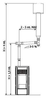
Fig. 3 - Pellet stove installation example
