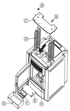
Fig. 42 - Cleaning the pipe unit, turbulators and lower compartment (lbis 11 / Idron 11)
