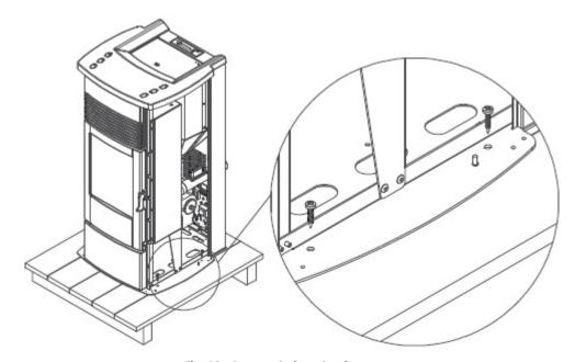
Fig. 13 - Removal of packaging screws
