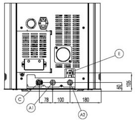
Fig. 18 - Plumbing connection
