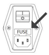
Fig. 44 - Fuse compartment
